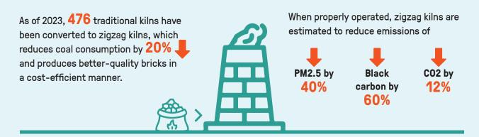
iv True zigzag technology includes four essential elements working in unison: zigzag chimney design, electric blowers/ air circulators, enhanced kiln insulation and fuel management. Interventions that do not include all four aspects may not see similar results to those reported.
